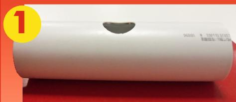
Drill the multilayer pipe with the specific cutter and smooth down the edges of the hole with rubbing paper
