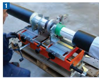
Perform the welding operation by following the instructions that are described in the technical catalogue. Before welding the second end, make sure that you introduced the heat-shrinking casing pipe still covered with the supplied film.
